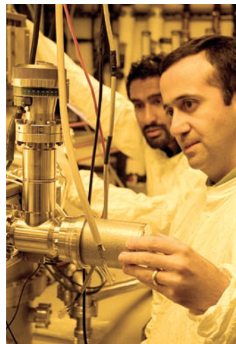
Shakouri and research assistant Rajeev Singh with the molecular beam epitaxy machine used to create nanostructured materials.
