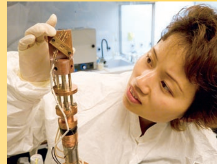
Graduate student Yan Zhang with a cryostat used to test thermoelectric materials over a range of temperatures, from near absolute zero to over 1,000 degrees Fahrenheit
