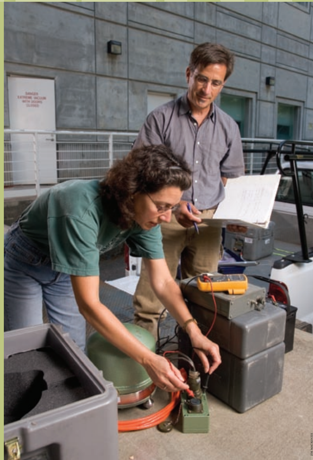
Prior to transport, professor of Earth and planetary sciences Susan Schwartz and colleague Dan Sampson inspect and pack the GPS and seismographic monitoring instruments they will be installing in Costa Rica.
