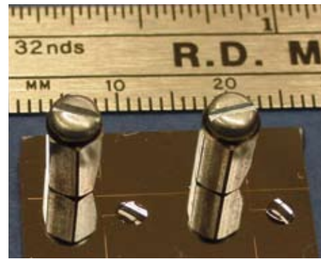
Atomic spectroscopy on a chip was achieved using this device, which features interconnected waveguides, rubidium vapor cells, and fiber-optical access.
