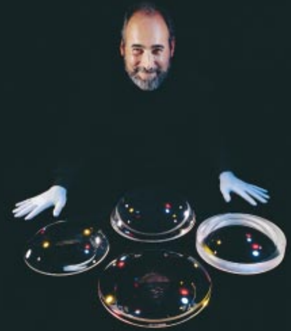
Optician David Hilyard used polishing wizardry to create these lenses for a camera in DEIMOS, including the world's largest polished crystal of calcium fluoride (rear, on table). Nine lenses, smoothed to within millionths of an inch, will focus light from galaxies onto a detector. The diagram below shows how light rays bend through the lenses.
